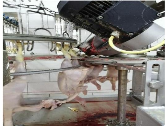
**Figure 40 :** Coupure des pattes (Photo originale, 2020)
