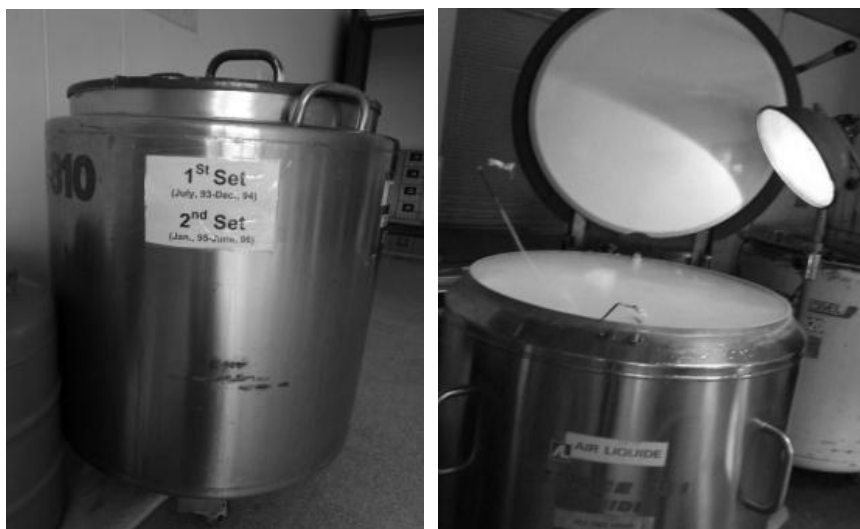
Fig. 3: A. Liquid nitrogen container for liquid nitrogen storage only B. LN 2 container for storage of semen doses.
