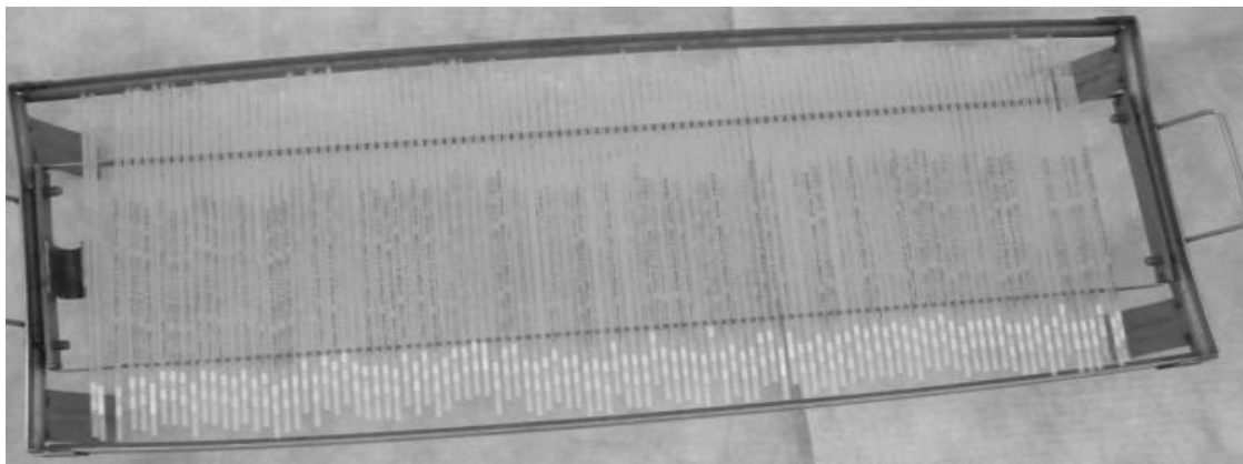
Fig. 8: Straws are spread over freezing rack
