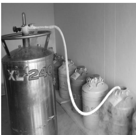
Fig.6: A. A funnel is placed into the neck before transfer of \text{LN}_2 B. \text{LN}_2 being transferred into the container.
