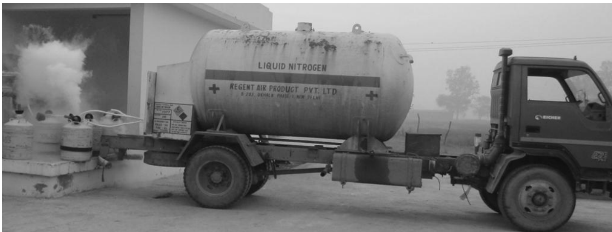
Fig.7: \text{LN}_2 being transferred from pressurized \text{LN}_2 container into Dewar container through transfer tube.
