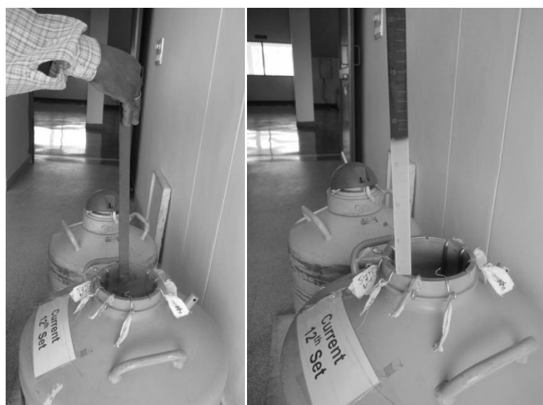
Fig. 9: Graduated dip sticks showing frost on the level of LN2 in the container.
