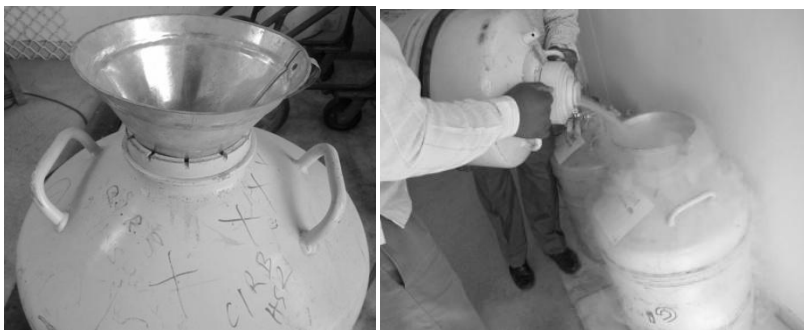
Fig.6: A. A funnel is placed into the neck before transfer of \text{LN}_2 B. \text{LN}_2 being transferred into the container.
