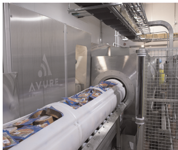
Figure 1 Horizontal HPP facility, processing deli meats. Photograph with permission from Avure Technologies and Maple Lodge Farms.
